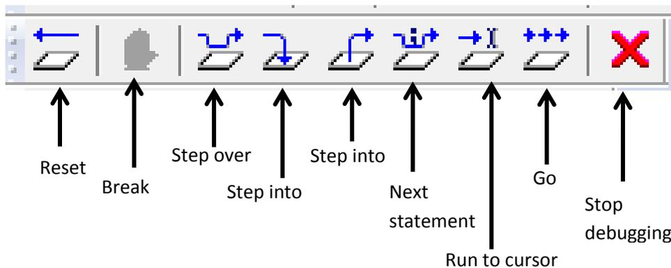
Figure 28. Toolbar for running code.
