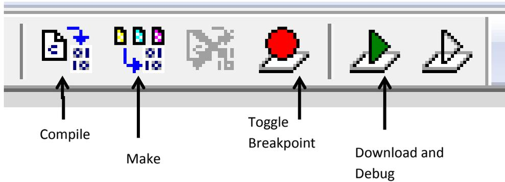
Figure 27. Toolbar for debugging and uploading code.
