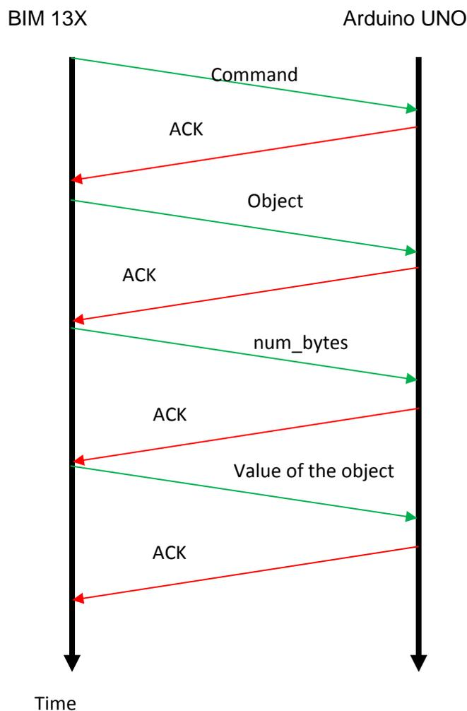
Figure 17. Sequence diagram of the communication protocol.
