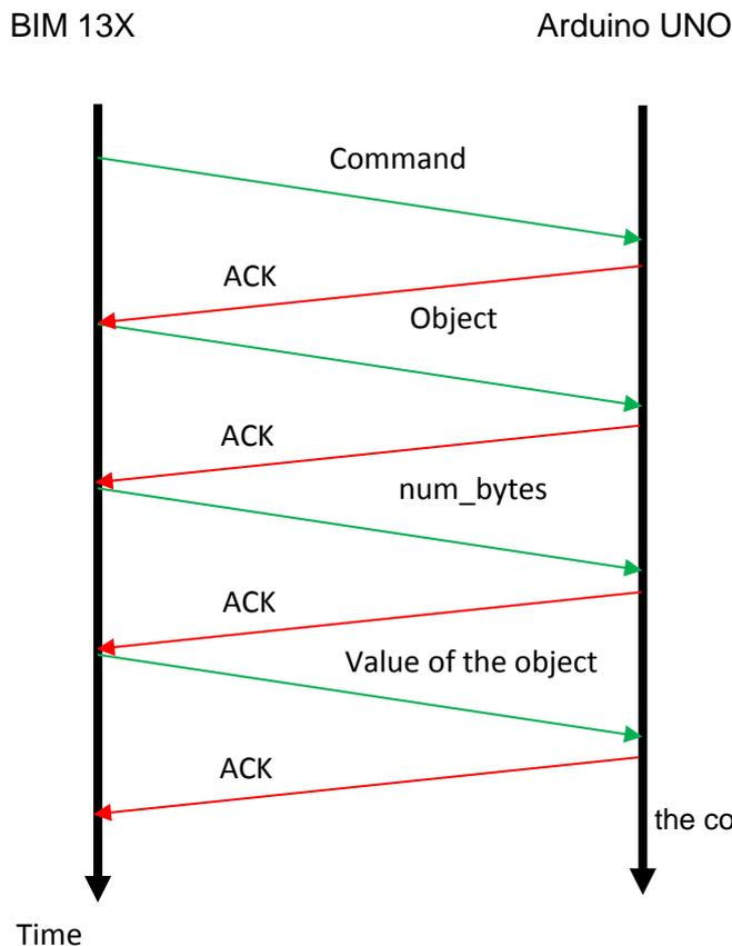
Figure 19. Sequence diagram of the communication protocol over FT12.
