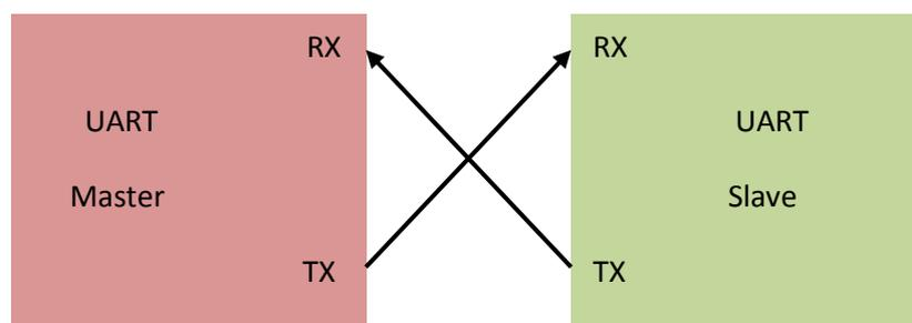
Figure 2. UART wire connection
