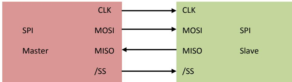
Figure 1: SPI wire connection
