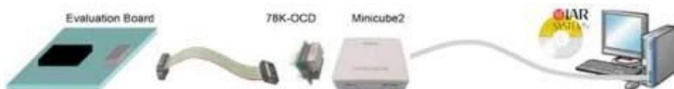
Figure 20. How to connect BIM system.
