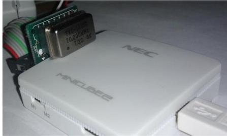
Figure 21. Oscillator mounted.
