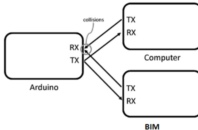
Figure 8. Colliding UART communication lines [16] pp.227
