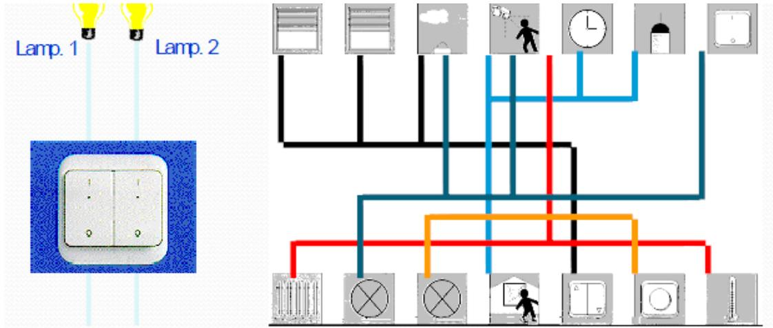
Figure 10. Conventional installation
