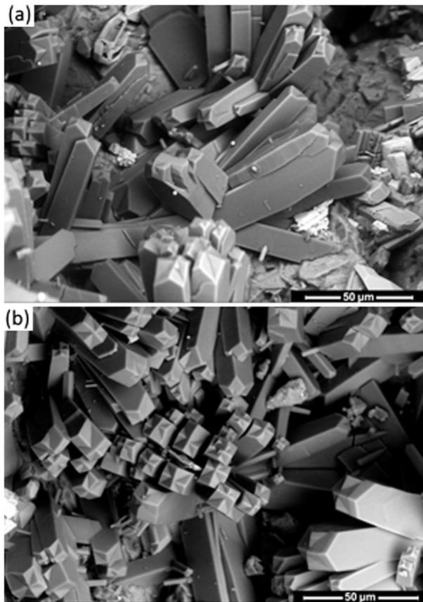
**Figure 6.** SEM Photograph of the zeolite occurrence. Radiating cluster of the zeolite crystal inside the cavities from the Arenas Negras volcano (a) and (b).
