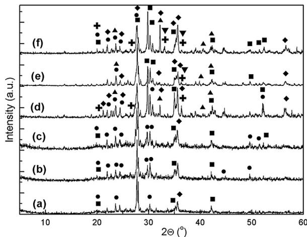
**Figure 4.** XRD diffractograms of different selected samples. (a) Pillow Lava (sub-sample 1); (b) Pillow Lava (sub-sample 2); (c) Pillow Lava (sub-sample 3); (d) The Arenas Negras volcano (TNFG1); (e) The Arenas Negras volcano (TNFG2); (f) The Arenas Negras volcano (TNFG3). Mineral assignment: (●) Plagioclase, (■) Pyroxene, (⊕) Hematite, (◆) Feldspar, (▲) Olivine and (▼) Goethite.
