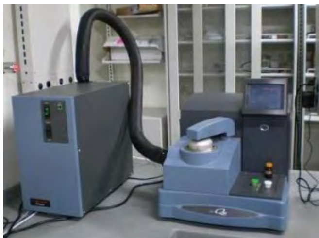
Figura 33. TA Instruments Thermo DSC modelo Q100
