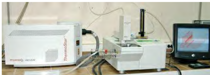
Figura 32. Mettler Toledo TGA/SDTA851e/SF/1100
