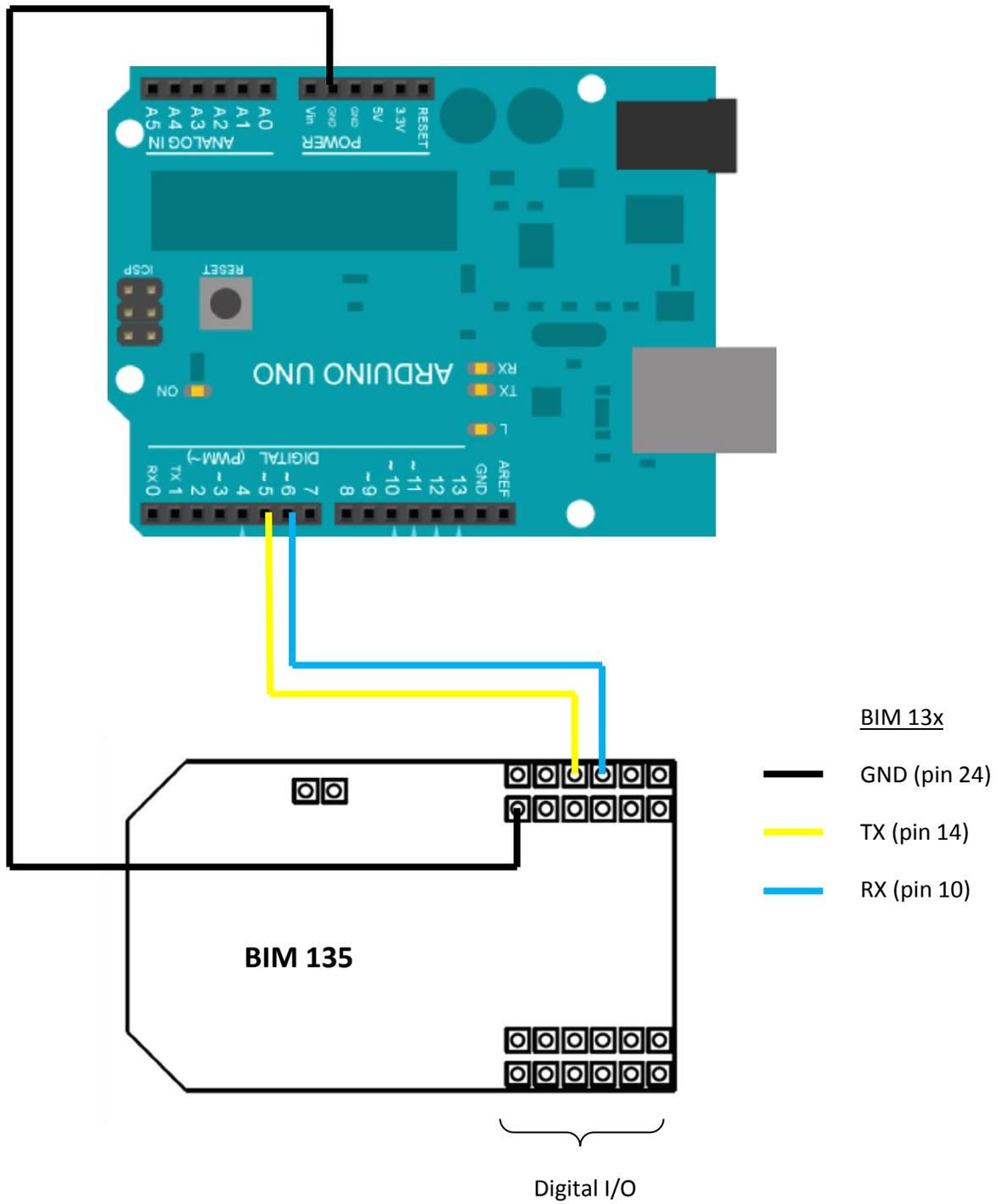
Figure 16. Wire connection between BIM board and Arduino
