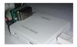
Figure 21. Oscillator mounted.
