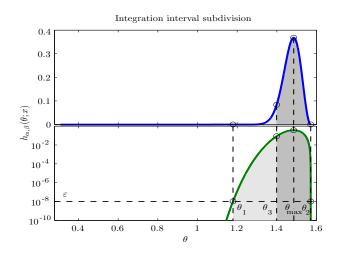
Figure 2: Subdivision of the integration interval in linear (top) and logarithmic scales (bottom). The maximum of the integrand  $(\theta_{max})$  and points for which  $h_{1.5,0.5}(\theta; x)$  croses a threshold  $\varepsilon$  ( $\theta_1, \theta_2$ ) are located. Then, a symmetric interval around  $\theta_{max}$  is determined ( $\theta_3$ ). In this example  $\alpha = 1.5$ ,  $\beta = 0.5$  and x = 6.
