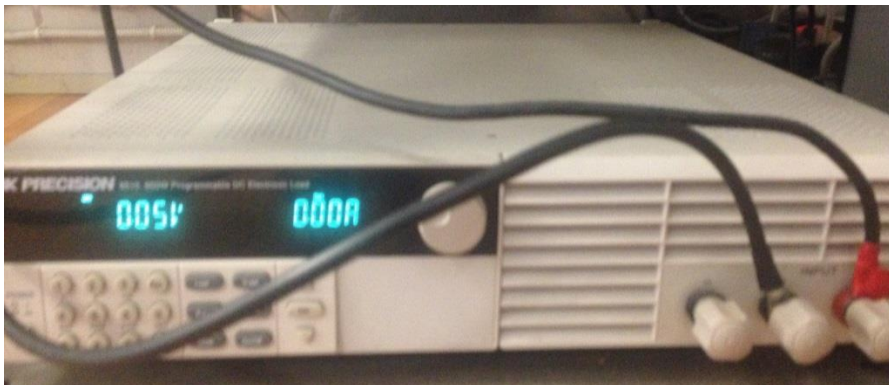
Figure 26: Test rig electronic load
