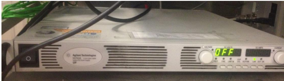
Figure 28: Test rig power supply
