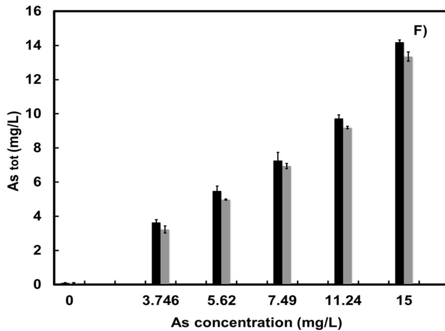
**Figure 4.3.** Total As(III) concentration (E) and total As(V) concentration (F) at the beginning and at the end of the experiments. Black bars represent the initial concentration. Grey bars represent the final concentration. The error bars represents the standard deviation of duplicates assays, or triplicates in the case of the control.
