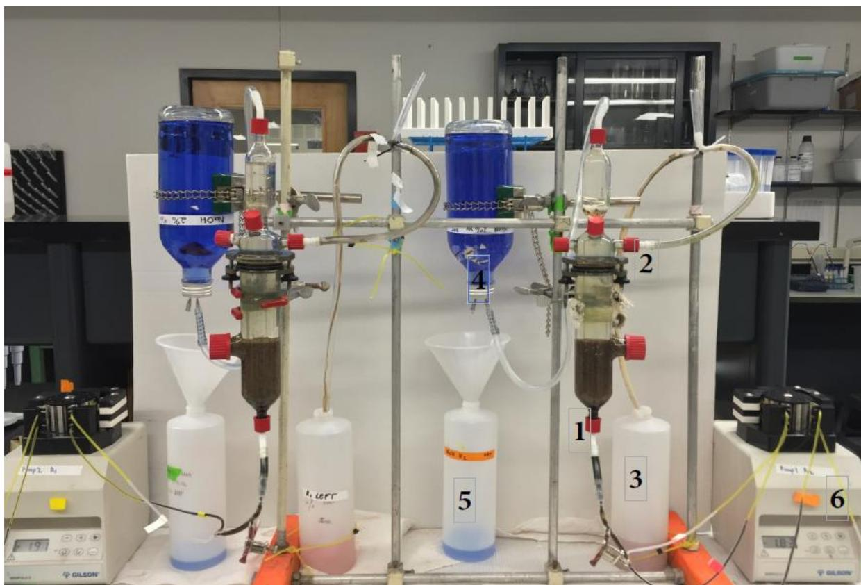
**Figure 3.2.** (1) Input Influent; (2) Output Effluent; (3) Collector Effluent; (4) NaOH dissolution to absorb  $\text{CO}_2$ ; (5) Collector of the NaOH dissolution displaced by  $\text{CH}_4$  produced in the bioreactor. (6) Pump.
