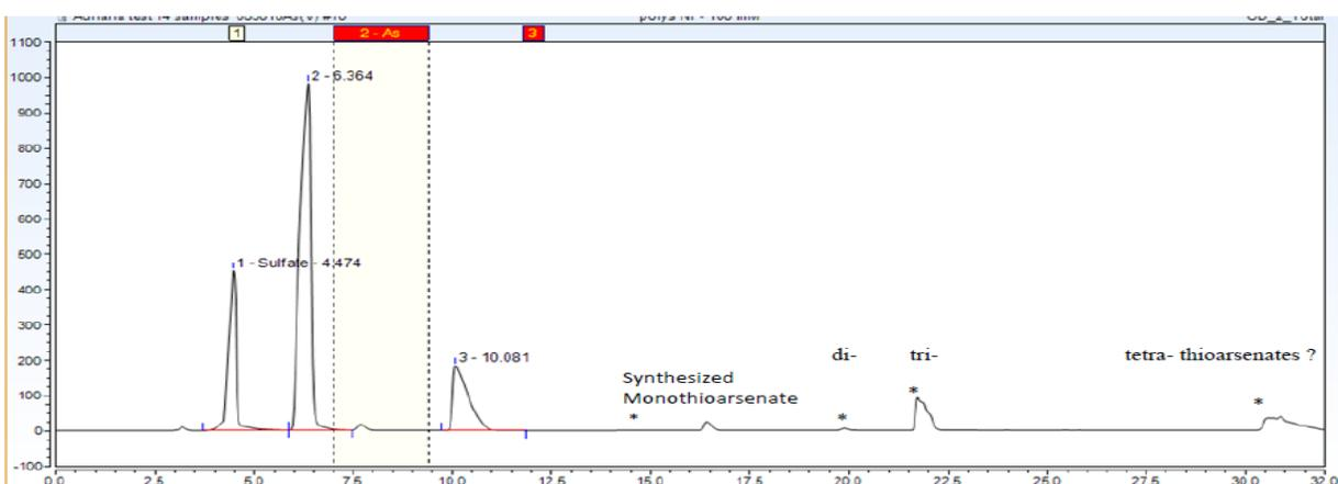
**Figure 4.15.** Separation of a mixture of thioarsenates (generated by mixing As(III) and sulfide) using ion chromatography. Axis Y (Intensity); Axis X (Time (min)).
