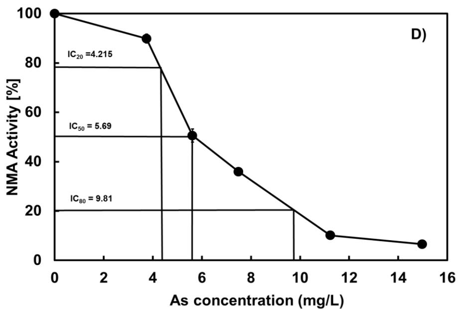
**Figure 4.2.** Normalized maximum methanogenic activity of the granular sludge as a function of the initial concentration of As(III) (C) and As(V) (D). The 20% (IC<sub>20</sub>), 50% (IC<sub>50</sub>) and 80% (IC<sub>80</sub>) inhibitory concentrations are shown on the figures. The error bars represent the standard deviation of duplicates assays, or triplicates in the case of the control.
