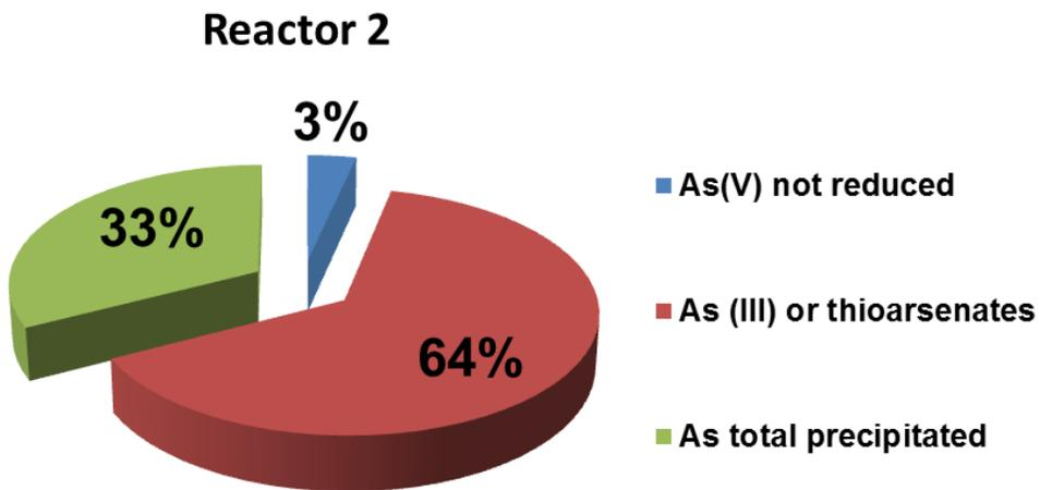
**Figure 4.12.** Arsenic speciation after treatment of an influent containing As(V) and different concentrations of sulfate in bioreactor 1 and 2.
