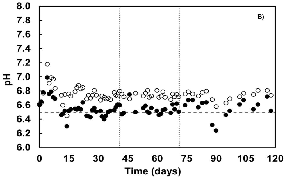
**Figure 4.7.** pH in the influent (●) and in the effluent (o) of reactor 1 (panel A) and reactor 2 (panel B). The horizontal black line represents the set point of the pH in the influent (6.5). The vertical dashed lines indicate the separation between the three stages in the reactor.
