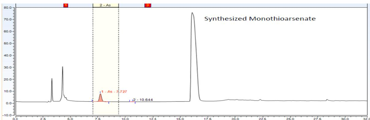
**Figure 4.14.** Monothioarsenate standard separation using ion chromatography. Axis Y (Intensity); Axis X (Time (min)).
