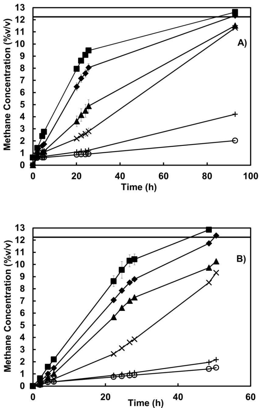
**Figure 4.1.** Methane (CH<sub>4</sub>) production in the experiments assessing the toxicity of different concentrations (expressed in mg/L) of As(III) (A) and As(V) (B): 0 (■); 3.75 (◆); 5.62 (▲); 7.5 (x); 11.24 (+); and 15 (o). The horizontal black line represents the maximum theoretical concentration of CH<sub>4</sub> that can be produced. The error bars represent the standard deviation of duplicates assays, or triplicates in the case of the control.
