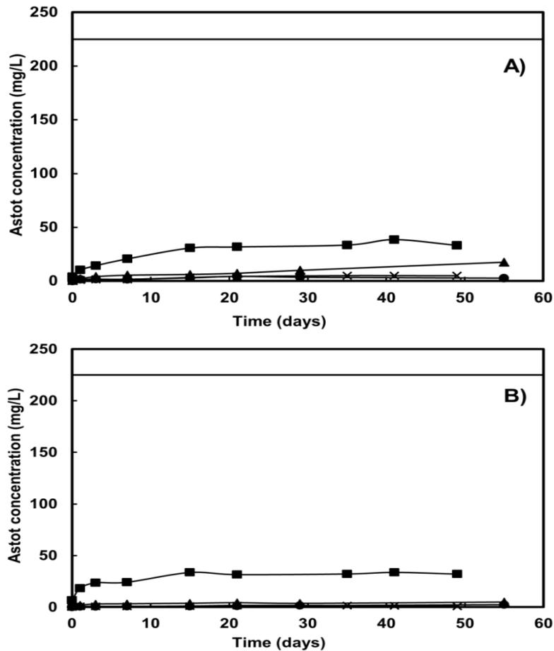
**Figure 4.17.** Dissolution of different ASM (225 mg/L as As) under aerobic conditions (A), and under anaerobic conditions (B) in batch assays at pH 8.45: Commercial orpiment (■), crushed orpiment (▲), arsenopyrite (x), realgar (●). The horizontal black line represents the maximum theoretical concentration of As that can be dissolved.
