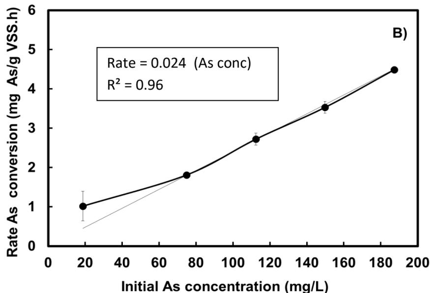
**Figure 4.5.** The rate of As(V) reduction to As(III) in Mahou anaerobic granular sludge incubated with at variable initial concentrations of As(V) with H<sub>2</sub> (8 psi) as electron donor. The error bars represent the standard deviation of duplicate assays. Linear fitting is represented in the graphic.
