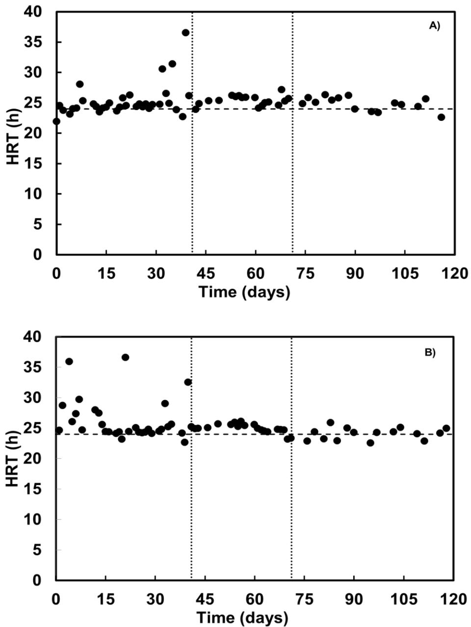
**Figure 4.6.** Hydraulic retention time (HRT) in reactor 1 (A) and reactor 2 (B). The horizontal black line represents the set point of the HRT (24 h). The vertical dashed lines indicate the separation between the three stages in the reactor.
