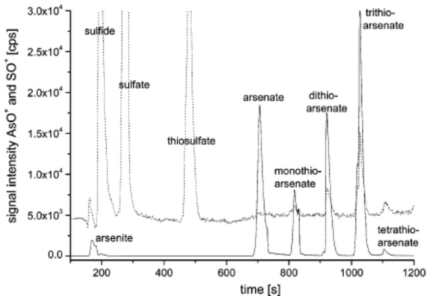
**Figure 4.16.** Chromatogram of an alkaline (pH 9, 90°C) geothermal water with high sulfide concentrations (3.7 mg/L) and a predominance of thioarsenates (solid line=  $\text{AsO}^+$ , dashed line =  $\text{SO}^+$ ). This chromatogram was obtained in a liquid chromatography system coupled to an ICP-MS [15].
