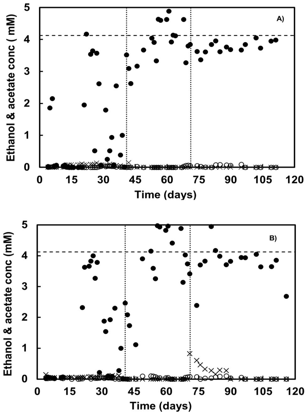
**Figure 4.8.** Transformation of ethanol and production of acetate in the reactors. (A) ethanol and acetate concentration in reactor 1; (B) ethanol and acetate concentration in reactor 2. (●) ethanol in the influent; (○) ethanol in the effluent; (x) acetate in the effluent. The horizontal black line represents the set point of the ethanol in the influent. The vertical dashed lines indicate the separation between the three stages in the reactor.
