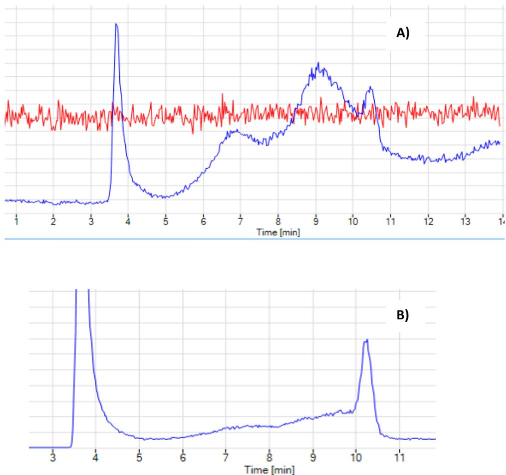
**Figure 4.13.** HPLC-ICP-MS chromatograms. (A) Monothioarsenate;(B) Effluent sample of reactor 2.
