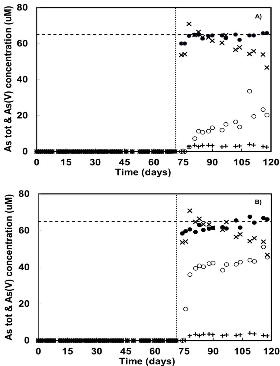
**Figure 4.11.** Total As and As(V) concentration in reactor 1 (A) and reactor 2 (B). (●) As total in the influent; (o) As total in the effluent; (x) As(V) in the influent; (+) As(V) in the effluent. The horizontal black line represent the set point of As total and As(V) in the effluent (65 µM). The vertical dashed lines indicate the beginning of the stage three in the reactor.
