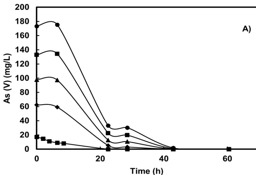
**Figure 4.4.** As(V) reduction to As(III) in Mahou anaerobic granular sludge using different initial As(V) concentrations (expressed in mg/L): 18.7 (■); 74.9 (◆); 112.4 (▲); 149.8 (■); and 187.3 (●). The error bars represent the standard deviation of duplicates assays.
