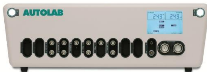
Figura 19. Potenciostato/galvanostato PGSTAT128 (Autolab Metrohm, Utrecht, Netherlands).
