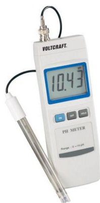
Figure 7. Typical pH sensor.
