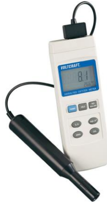
Figure 8. Typical DO sensor
