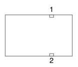
$$S_1*V_1 = S_2V_2 \\ 308cm^2*V_1 = 4.7cm^3/s \\ V_1 = 0.01526cm/s \\ P_1 + \frac{1}{2}\rho V_1 + \rho gh = P_2 + \frac{1}{2}\rho V_2 \\ P_1 = 10.2 \ KPa$$
