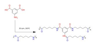
Figure 1. Molecular structure of star-shape polyamide
