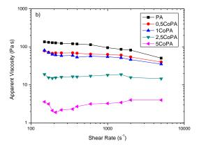
**Figure 2.** Apparent viscosity of star-shape polyamides by capillarity rheometry versus shear rate: a) 230°C and b) 260°C
