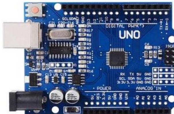
Figura 3.2.1.1 -Arduino UNO R3 ATmega328P CH340G. Fuente: <https://www.makerlab-electronics.com/product/arduino-uno-r3-atmega328p-ch340g/>
