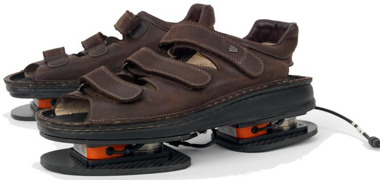
Figura 7.30: XSENS ForceShoe<sup>TM</sup> [7].
