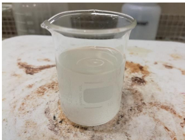
FIGURE 18. IMAGE OF NON SPINNABLE SOLUTION WITH PRECIPITATE.
