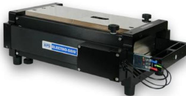
The APS 400 ELECTRO-SEIS® shaker is a longstroke, electrodynamic force generator specifically designed to be used alone or in arrays for studying dynamic response characteristics of various structures. It finds use in modal excitation of complex structures, particularly when low frequencies are required. Furthermore it can be used for low frequency vibration testing of components and assemblies.
