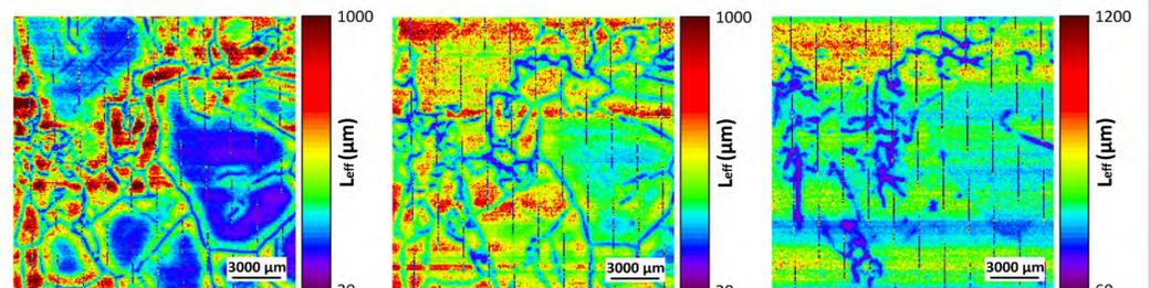
L<sub>eff</sub> increases from A to C. In sample A the diffusion length is severely reduced inside the grains, while it increases around the defects because of the impurity depletion around them.
