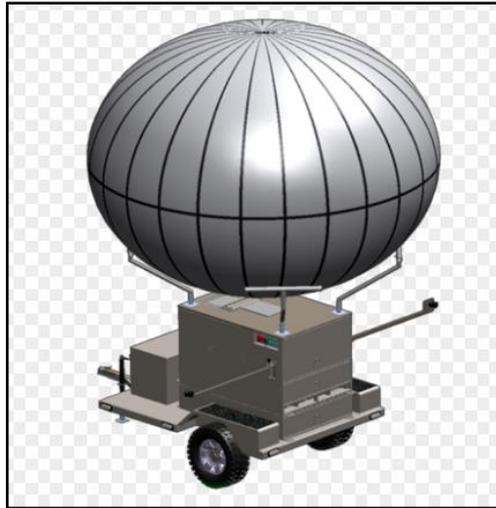
*Figura 3: Winch Aerostat Swal Platform*<sup>3</sup>
