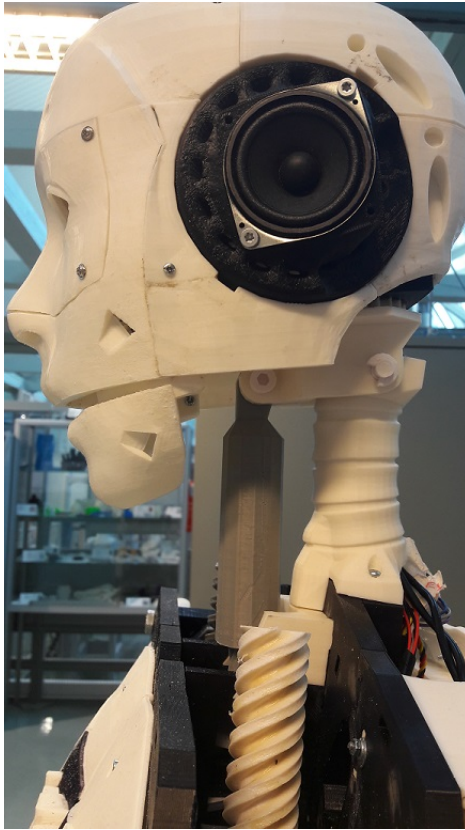
Figure 6.12: Fully Reassembled and connected head connected to the body with two bolts
