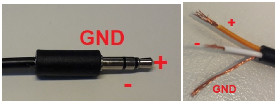
Figure 6.9: Sections of an AUX wire
