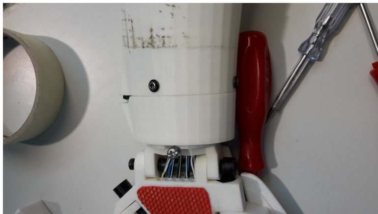
Figure 6.14: Closed wrist assembly
