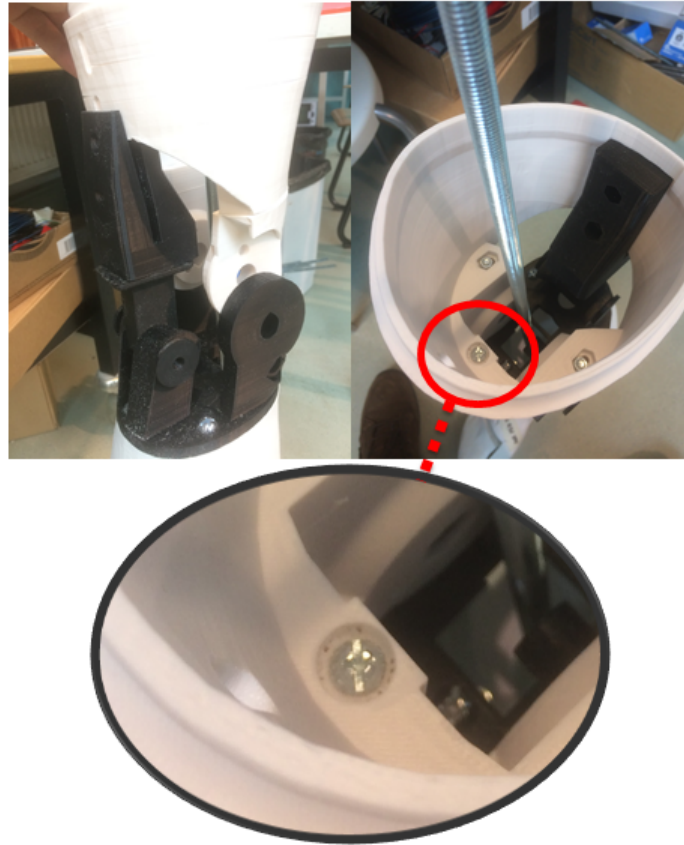
Figure 6.55: Assembling the knee to the thigh
