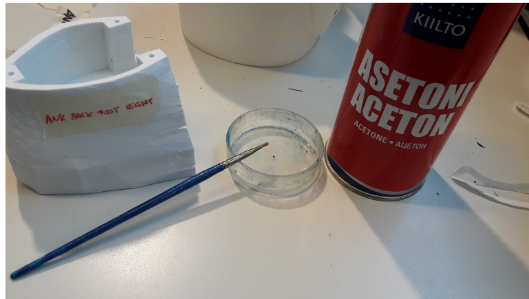
Figure 6.38: Acetone used to repair damaged parts
