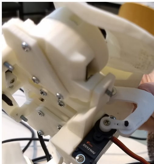
Figure 6.2: Implementation of the servo DS929HV for the y-movement of the eyes
