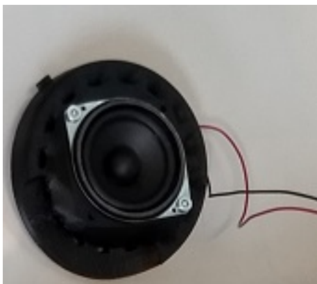
Figure 6.8: Loudspeaker with ground wire (black) and signal wire (red)
