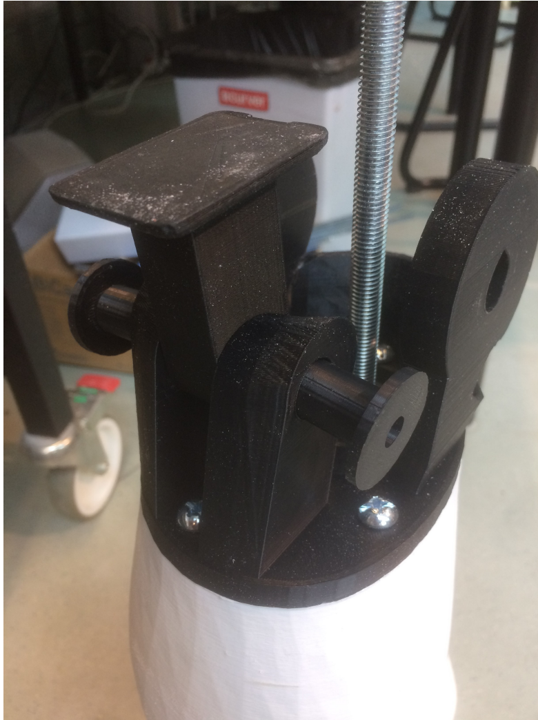
Figure 6.54: Knee connection with the " KneeClampRightV1 " and the " KneeSmallBoltsV1 "
