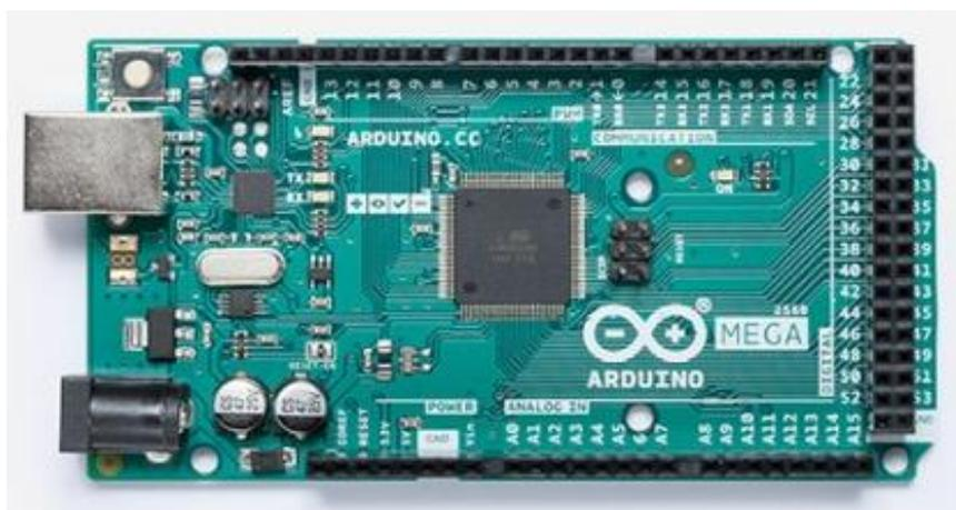
Figura 36. Arduino Mega 2560 rev3
