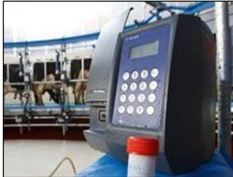
Figura 21: Cell counter DCC. Fuente: DeLaval.
