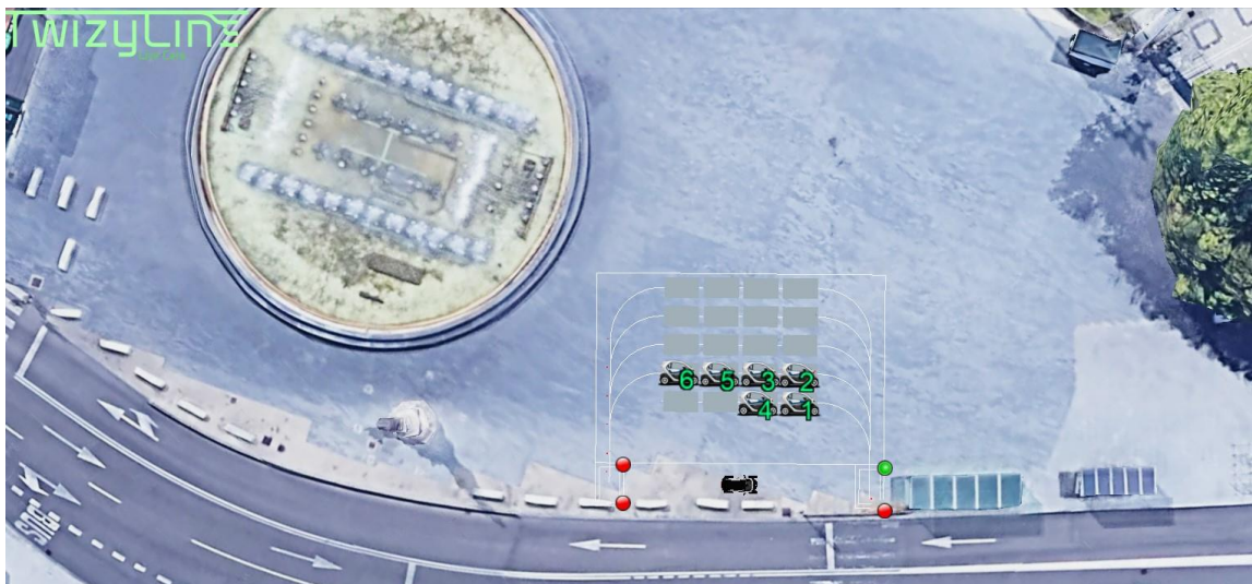
Figure 62. Barrier 3 opens (green point) because the Twizy number 2 must drive to the pick-up zone.
