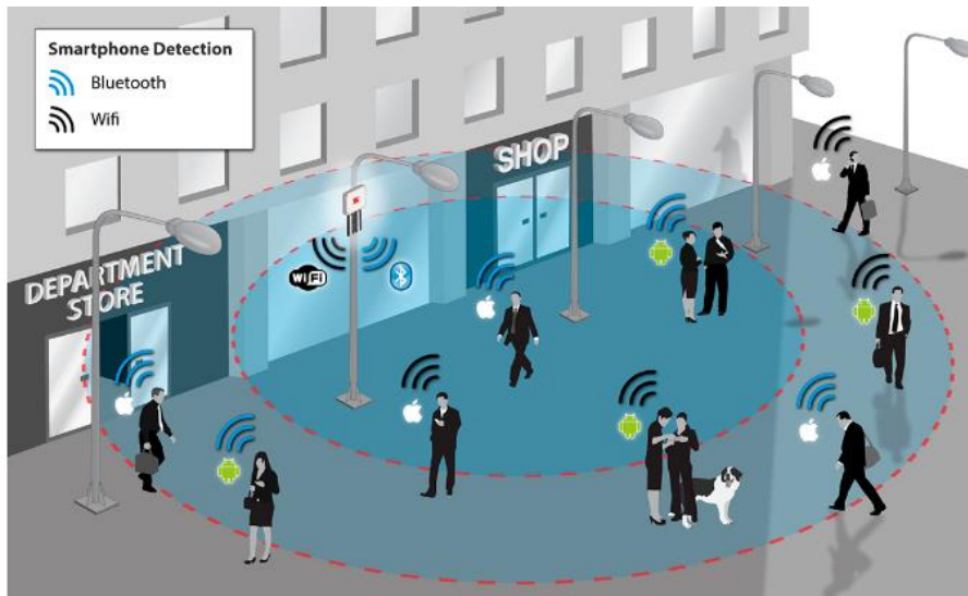
Figure 9. Meshlium Scanner to measure the number of people gather in a defined area [32]
