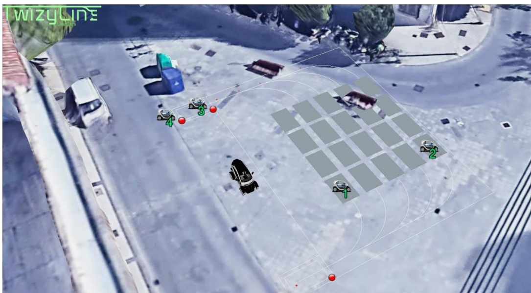
Figure 51. TwizyLine parking from Plaza Portugaleta. Barrier 1 does not open because the leaving zone is occupied.
