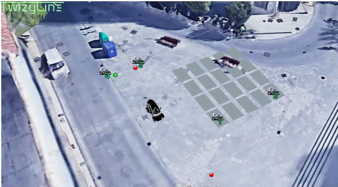
Figure 52. Barrier 1 is enabled to open now, as the leaving zone is empty and the barrier 2 is closed.
