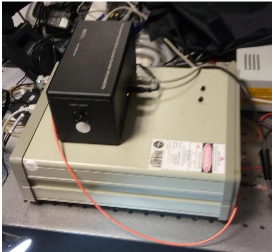
*Figure 11. CompassT Spectrometer (dark colored) on top of the laser box (light colored).*
