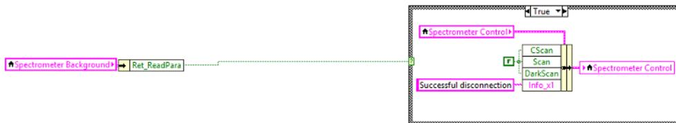
Figure 36. LabVIEW disconnection phase of the RAD1 spectrometer.
