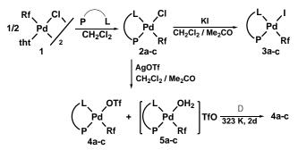
Scheme 1. Synthesis of the complexes used in this work. Rf = 3,5-C<sub>6</sub>Cl<sub>2</sub>F<sub>3</sub>
