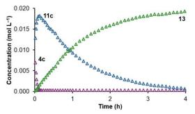
Fig. 13. <sup>19</sup>F NMR monitoring of the reaction between [Pd(Rf)(OTf){PPh<sub>2</sub>(bzN)}] (4c) and PhC=CSnBu<sub>3</sub> (9) (Pd:Sn = 1:20) in THF at 313 K.
