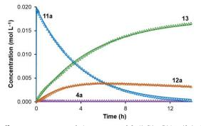
Fig. 5.  $^{19}F$  NMR monitoring of the reaction of [Pd(Rf)(OTf)(dppe)] (4a) with PhC=CSnBu<sub>3</sub> (9) (Pd:Sn = 1:20) at 313 K. Continuous lines are the result of COPASI fitting.
