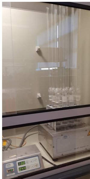
FIGURE 16 | Residual P extraction with \text{HClO}_4 in the digestion block. Photos by ©R.C. Martín-Sanz.
