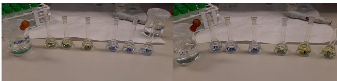
FIGURE S9.3.1. | Adjustment of pH. (a) Turn from colorless to yellow by adding 5 M NaOH. (b) Turn from yellow to colorless by adding 1 M HCl. Photos by ©R.C. Martín-Sanz.
