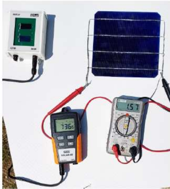
Fig. 10 Irradiances and short circuit current measured on field test.
