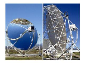
Figure 17: Eurodish (Stirling dish) at Almeria solar platform (Ciemat) [36].
