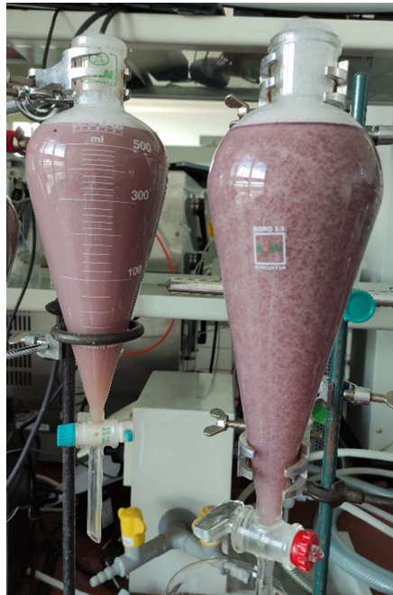
Figure 4-4: WW poured in the separatory funnel before separation of flocs.
