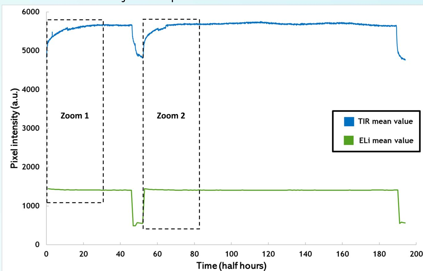
Zoom zones in upper graph, showing module heat ups due to the current injection.
