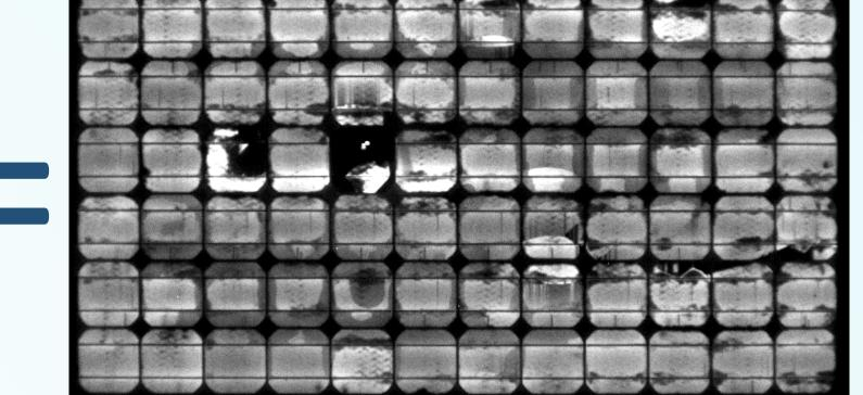
A detailed analysis was performed in order to see the defects induced by current injection.
