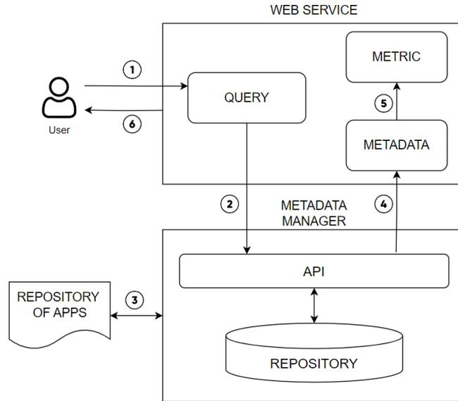
**Fig. 3.** System data flow.
