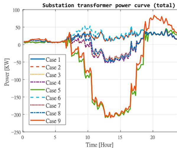
Figure 5. Substation transformer power curve for each case.
