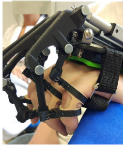
Fig. 12. Exoskeleton placed in the hands of two spastic patients during tests at the University Clinical Hospital (Valladolid, Spain).
