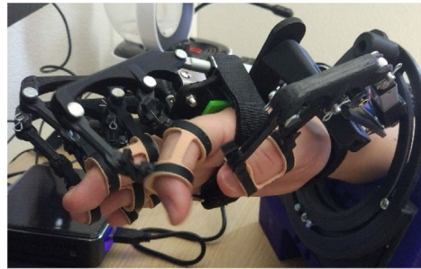
Fig. 12. Exoskeleton placed in the hands of two spastic patients during tests at the University Clinical Hospital (Valladolid, Spain).
