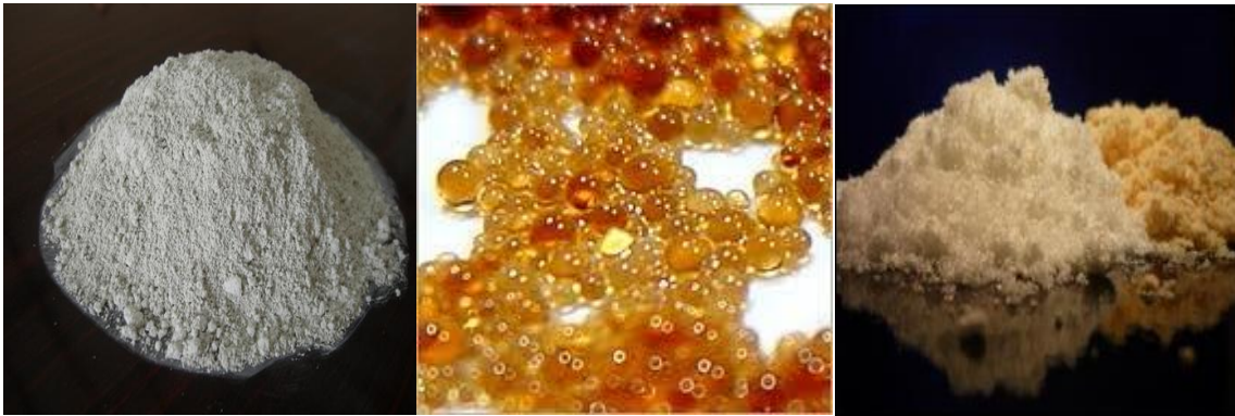
Figure 21-Different acid catalyst (from left to right): Zeolite, Ion exchange resin and super acid fibrous catalyst
