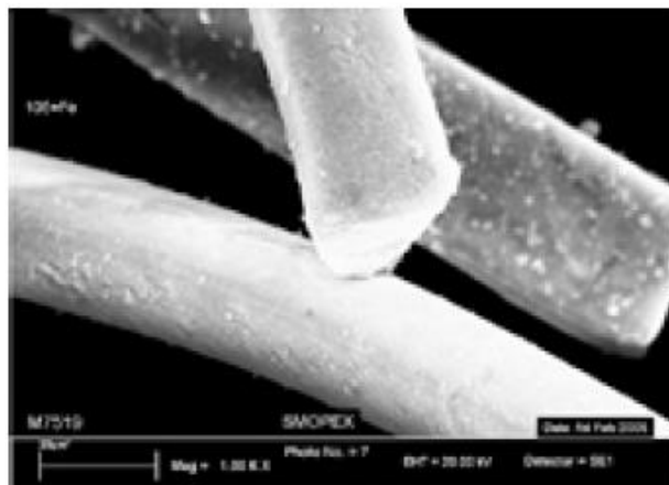
Figure 33-Sulfonic functional group of Smopex-101 (left) and SEM picture of the fibers of Smopex-101 (right)
