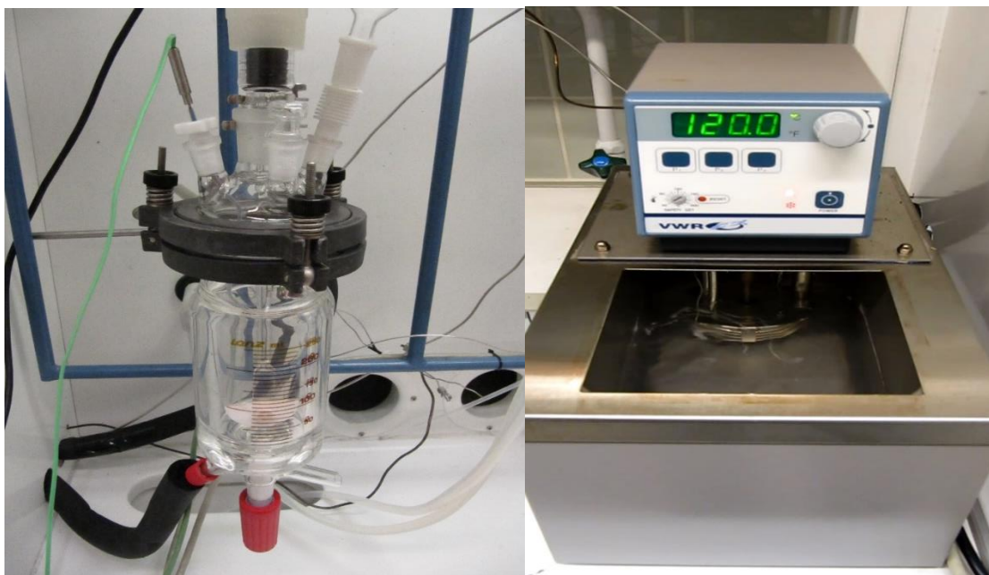
Figure 30-Reactor set up and Silicone oil bath
