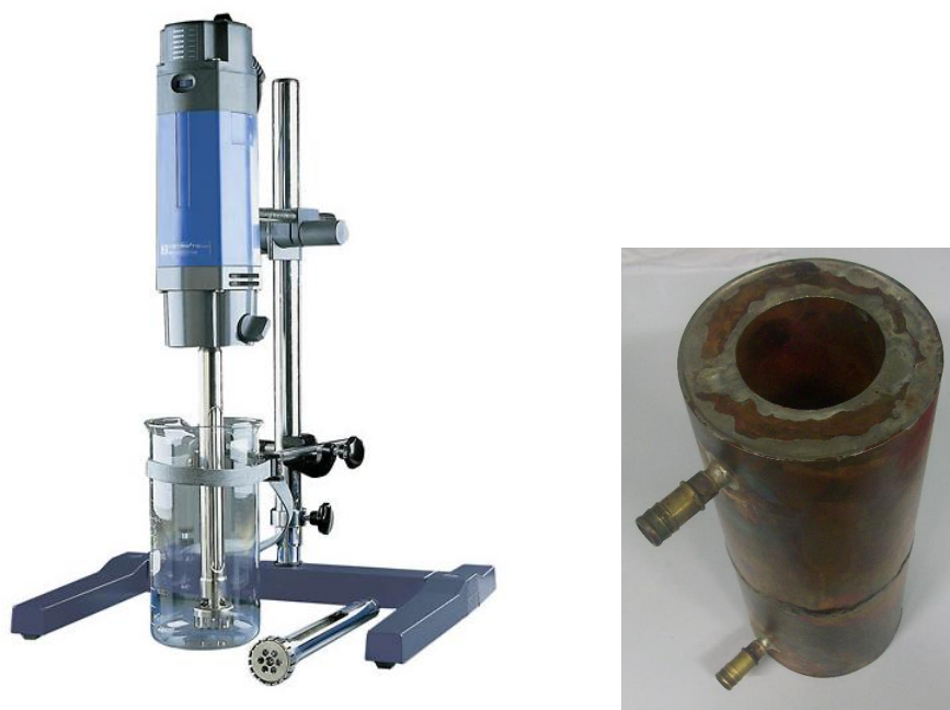
Figure 4. 3 IKA® T 50 ULTRA-TURRAX® (left) [75] and jacketed cooper container (right)
