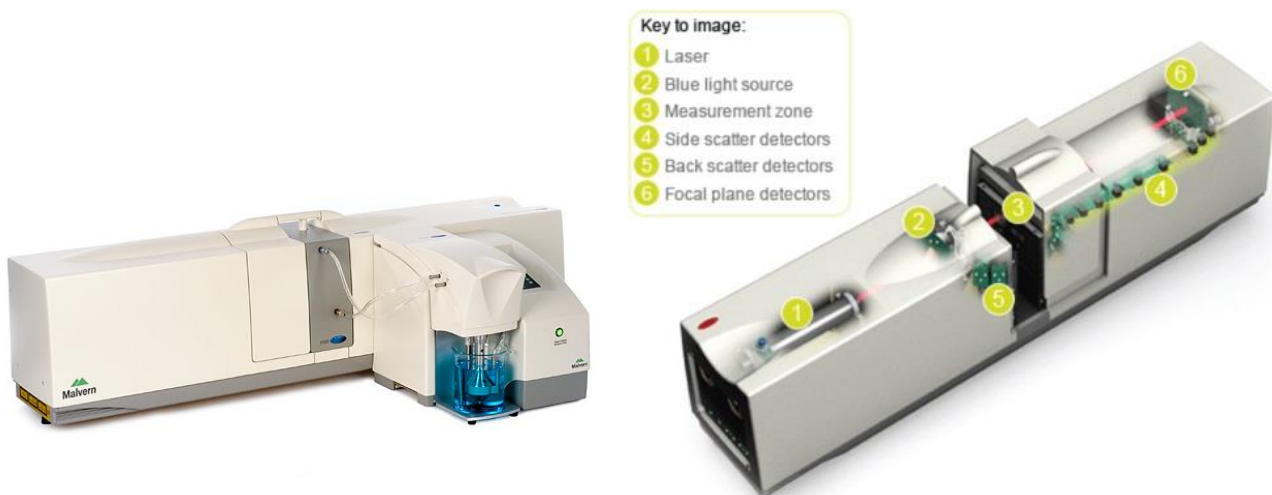
Figure 4. 5 Mastersizer 2000 from Malvern with wet module (left) [78] and a schematic of how laser diffraction technique is placed inside (right) [81]
