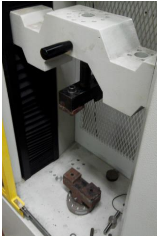
Illustration 70 The final installation of the fixture in the traction machine.
