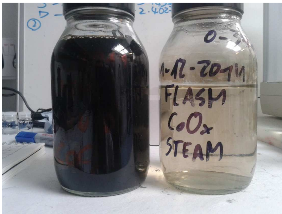
Figure 26. Samples of the liquid and vapour collected during the synthesis of cobalt oxide
