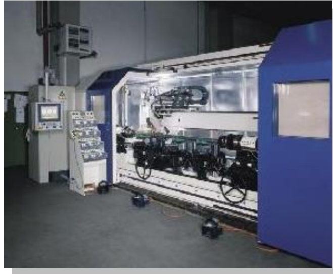
Figura 25. Equilibradora SCHENCK KHGW 20-B
