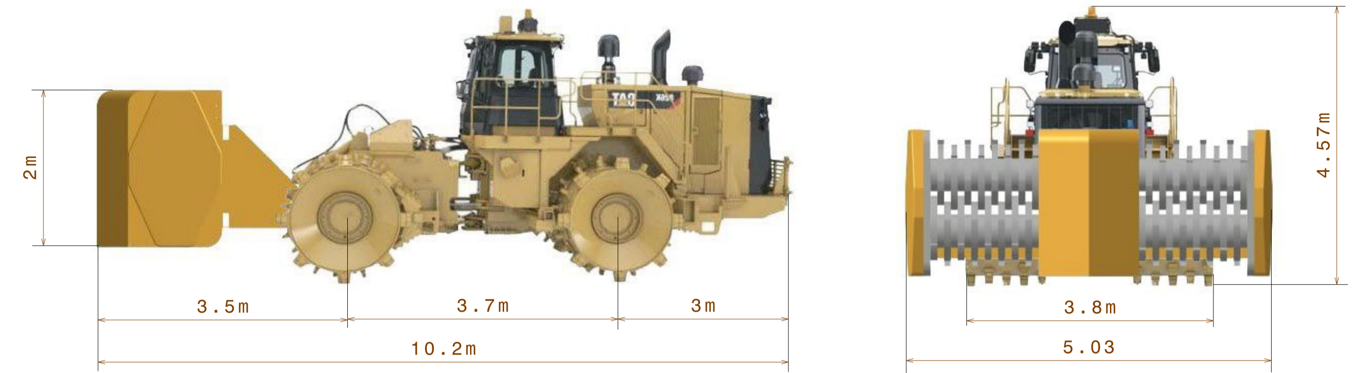
Right and front views of waste compactor with the shredder attachment Scale: 1:50
