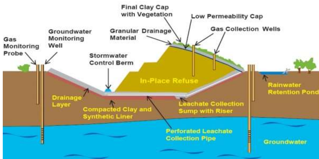
Figure 1.1-1: Elements in controlled landfills 3
