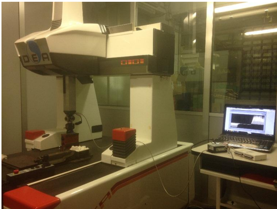
Illustration 65 Implementation of Fiberoptic sensor into CMM
