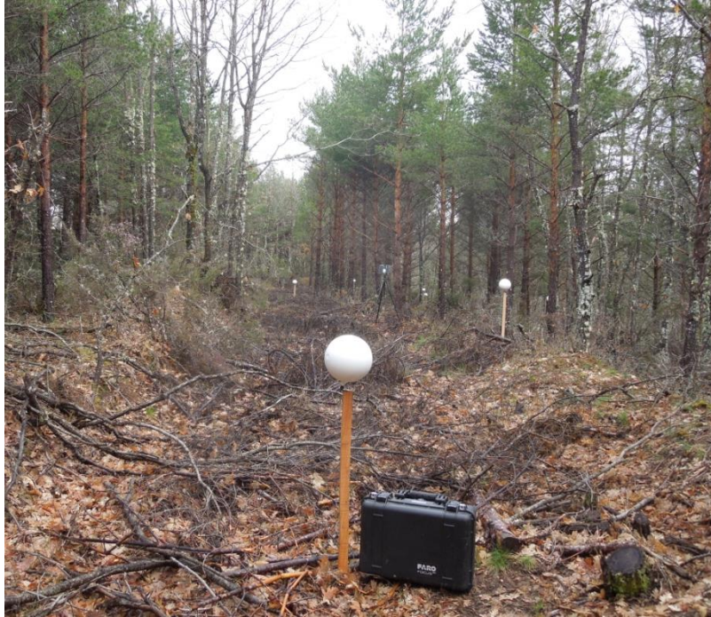
Figure 2. The five georeferencing points were marked by using White spheres needed for later 3D reconstruction and in order to distinguish them from other they were marked as in this case with a luggage.
