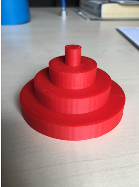
Figure 48: Metrological Specimen: Distance Between Planes
