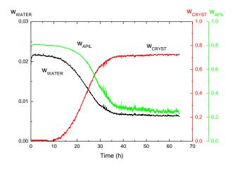
Figure 39. Evolution of concentration of crystals, water and API for reference sample ( $w_{NIF}$  80%,  $40^{\circ}$ C, 75%RH)
