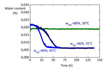
Figure 34. Evolution of water content along temperature for w<sub>NIF</sub> 80% and 75%RH
