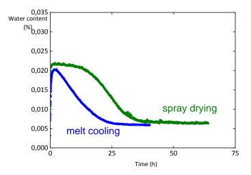
Figure 37. Evolution of water content along the method to prepare the formulation for  $w_{NIF}$  80%, 40°C and 75%RH
