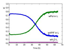
Figure 52. Concentration of components in the liquid phase for sample w<sub>NIF</sub> 0.75, 40°C, 75%RH
