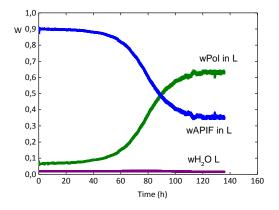
Figure 60. Concentration of components in the liquid phase for sample w<sub>NIF</sub> 0.90, 30°C, 75%RH
