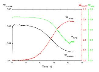
*Figure 51. Evolution of concentration of crystals, water and API for sample w<sub>NIF</sub> 0.85, 40°C, 75%RH* 59
