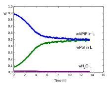
Figure 70. Concentration of components in the liquid phase for sample  $w_{NIF}$  0.90 in Resomer R203s, 40°C, 75%RH
