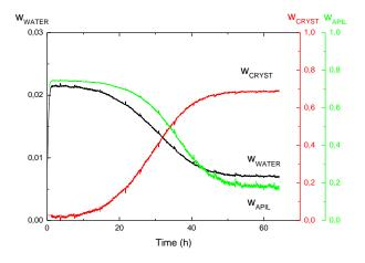
Figure 53. Evolution of concentration of crystals, water and API for sample w<sub>NIF</sub> 0.75, 40°C, 75%RH
