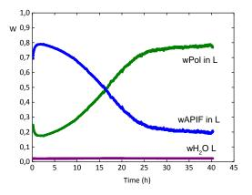
*Figure 54. Concentration of components in the liquid phase for sample w<sub>NIF</sub> 0.80, 40°C, 75%RH by melting-cooling*
