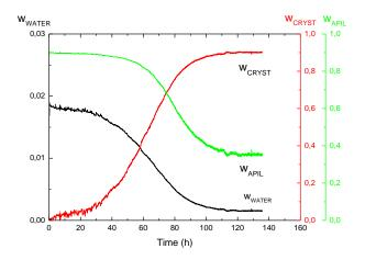
Figure 61. Evolution of concentration of crystals, water and API for sample w<sub>NIF</sub> 0.90, 30°C, 75%RH
