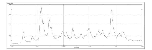
Figure 4. PXDR pattern of a recrystallized sample (w<sub>NIF</sub> 80%, PVAC350, 40°C, 75%RH) obtained after the suspension balance experiment
