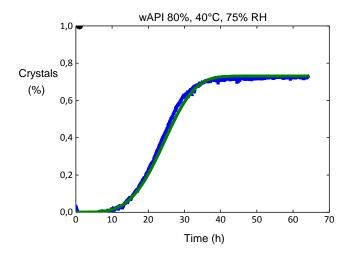
Figure 42. Coupling of the experimental curve and Avrami theoretical curve
