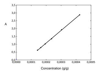
Figure 76. Calibration curve of NIF at 276 nm in acetonitrile
