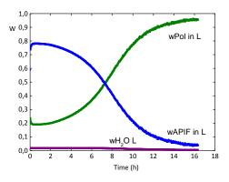
Figure 72. Concentration of components in the liquid phase for sample  $w_{NIF}$  0.80 in Resomer R203s, 40°C, 75%RH
