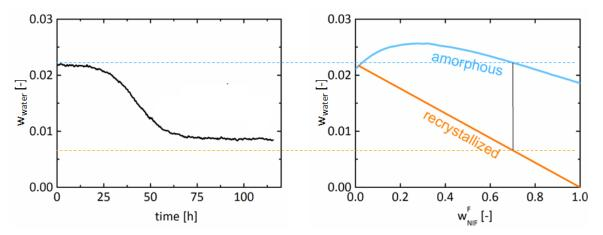
Figure 10. Behavior of water content and phases during crystallization for a w<sub>NIF</sub> 70% [10]
