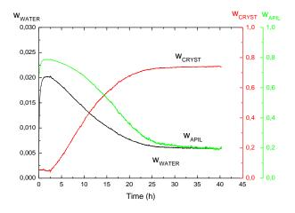
*Figure 55. Evolution of concentration of crystals, water and API for sample w<sub>NIF</sub> 0.80, 40°C, 75%RH by melting-cooling*
