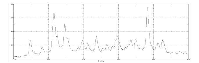
Figure 41. PXDR pattern of crystalline state of sample w<sub>NIF</sub> 80%, 40°C and 75%RH
