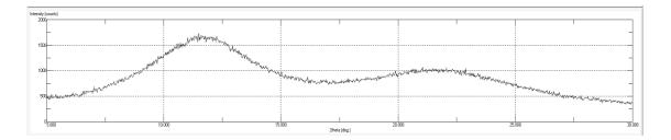
Figure 3. PXDR pattern of an amorphous sample (w<sub>NIF</sub> 70%)
