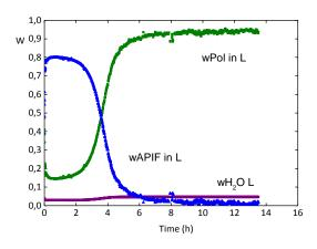
Figure 56. Concentration of components in the liquid phase for sample w<sub>NIF</sub> 0.80, 40°C, 90%RH
