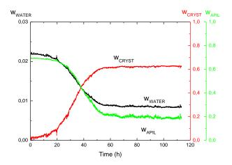
Figure 49. Evolution of concentration of crystals, water and API for sample w<sub>NIF</sub> 0.70, 40°C, 75%RH
