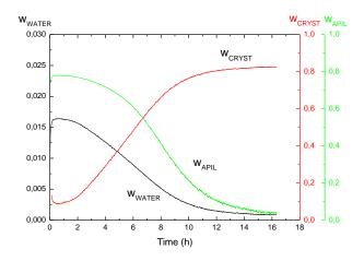
*Figure 73. Evolution of concentration of crystals, water and API for sample w<sub>NIF</sub> 0.80 in Resomer R203s, 40°C, 75%RH*
