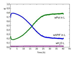
Figure 74. Concentration of components in the liquid phase for sample  $w_{NIF}$  0.70 in Resomer R203s, 40°C, 75%RH
