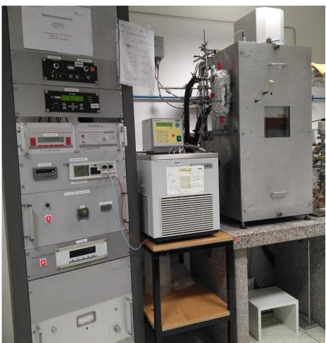
Figure 20. Suspension balance experimental installation
