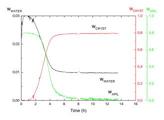
Figure 57. Evolution of concentration of crystals, water and API for sample w<sub>NIF</sub> 0.80, 40°C, 90%RH
