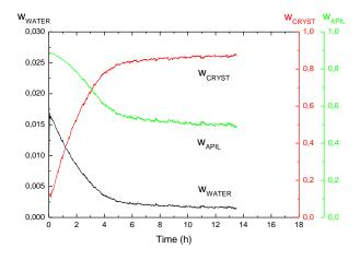
*Figure 71. Evolution of concentration of crystals, water and API for sample w<sub>NIF</sub> 0.90 in Resomer* R203s, 40°C, 75%RH
