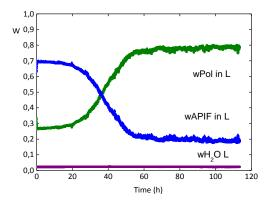
Figure 48. Concentration of components in the liquid phase for sample w<sub>NIF</sub> 0.70, 40°C, 75%RH
