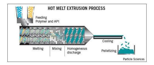
Figure 2 Hot melt extrusion process [7]
