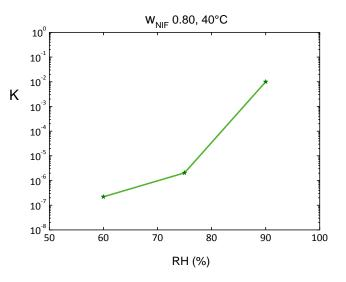
Figure 44. K coefficient behavior with relative humidity
