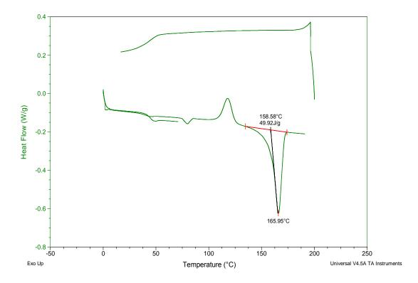
Figure 5. DSC thermogram of NIF/PVAC (w<sub>NIF</sub> 70%, PVAC, 40°C, 75%RH)
