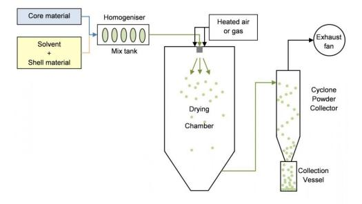
Figure 1. Scheme of spray drying method [6]
