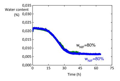
*Figure 30. Overlap of the two independent water sorption measurements obtained for* w<sub>NIF</sub>=0.80 *at 40* °C, 75% RH to check the reproducibility of the experiments
