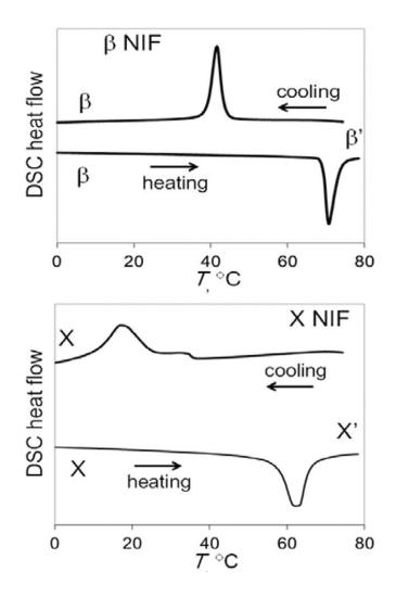
Figure 17. Behavior of the two polymorphs on heating and cooling [23]
