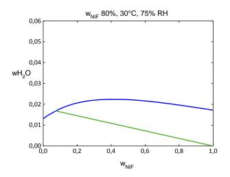
Figure 29. Sorption diagram for sample w<sub>NIF</sub> 80%, 30°C, 75°RH
