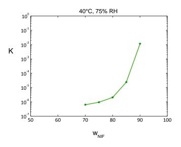
Figure 43. K coefficient behavior with API weight fraction
