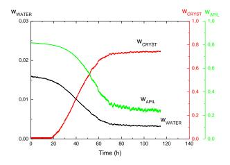
Figure 59. Evolution of concentration of crystals, water and API for sample w<sub>NIF</sub> 0.80, 40°C, 60%RH
