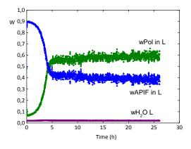
Figure 46. Concentration of components in the liquid phase for sample w<sub>NIF</sub> 0.90, 40°C, 75%RH
