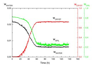
Figure 65. Evolution of concentration of crystals, water and API for sample w<sub>NIF</sub> 0.80, 35°C, 75%RH
