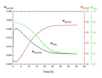
*Figure 75. Evolution of concentration of crystals, water and API for sample w<sub>NIF</sub> 0.70 in Resomer R203s, 40°C, 75%RH*
