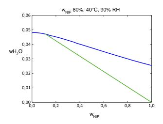
Figure 27. Sorption diagram for sample w<sub>NIF</sub> 80%, 40°C, 90°RH
