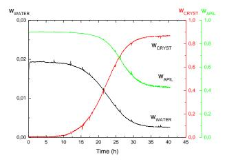
Figure 63. Evolution of concentration of crystals, water and API for sample w<sub>NIF</sub> 0.90, 35°C, 75%RH
