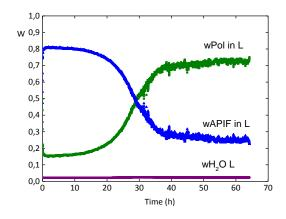
Figure 38. Concentration of compounds in the liquid phase for reference sample ( $w_{NIF}$  80%, 40°C, 75%RH)
