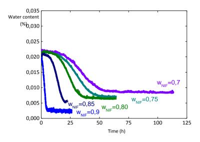
Figure 31. Evolution of water content along the weight fraction
