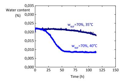
Figure 35. Evolution of water content along temperature for w<sub>NIF</sub> 70% and 75%RH
