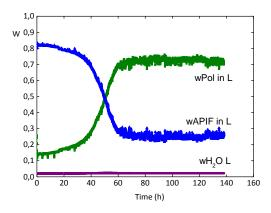
Figure 64. Concentration of components in the liquid phase for sample w<sub>NIF</sub> 0.80, 35°C, 75%RH
