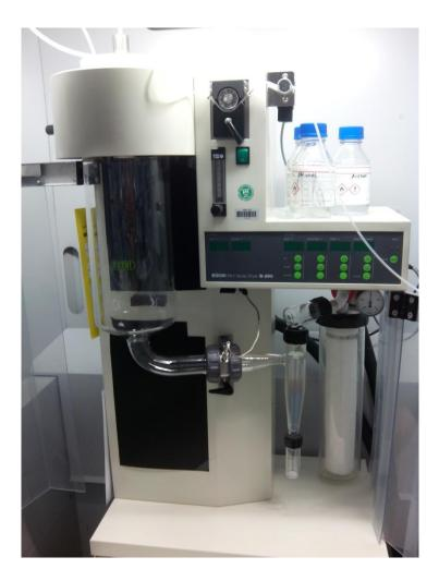
Figure 19. Büchi Mini Spray Dryer B-290 experimental installation
