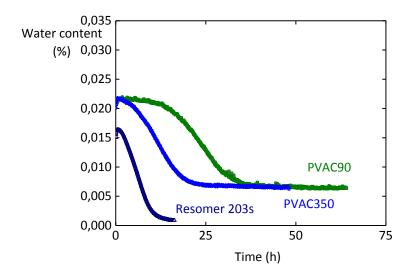
Figure 36. Evolution of water content along polymer for w<sub>NIF</sub> 80%, 40°C and 75%RH
