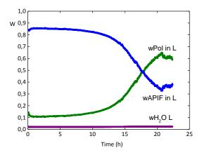
Figure 50. Concentration of components in the liquid phase for sample w<sub>NIF</sub> 0.85, 40°C, 75%RH
