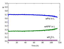
Figure 68. Concentration of components in the liquid phase for sample w<sub>NIF</sub> 0.70, 35°C, 75%RH
