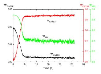
Figure 47. Evolution of concentration of crystals, water and API for sample w<sub>NIF</sub> 0.90, 40°C, 75%RH
