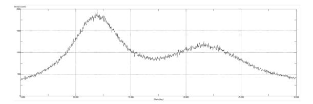
Figure 40. PXRD pattern of amorphous state of sample w<sub>NIF</sub> 80%
