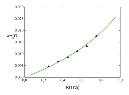
Figure 24. Fitting of the experimental and VLE NIF curves [25]
