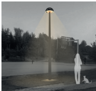
Pole top contains both functional and ambience light. Functional light is separated into 3 modules. Different light intensity levels can be arranged in those modules while assembly in order to answer different needs of the area like lighting courts or lighting different gathering areas.
