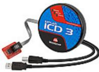
MPLAB® ICD 3 In-Circuit Debugger System is Microchip's most cost effective high-speed hardware debugger/programmer for Microchip Flash Digital Signal Controller (DSC) and microcontroller (MCU) devices. It debugs and programs PIC® Flash microcontrollers and dsPIC® DSCs with the powerful, yet easy-to-use graphical user interface of MPLAB Integrated Development Environment (IDE).
