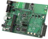
The PIC24FJ256DA210 Development Board is a low cost and efficient development board to evaluate the features and performance of the PIC24FJ256DA210 with integrated graphics, mTouch™ and USB. This board is an ideal platform for developing graphical human interface applications.
