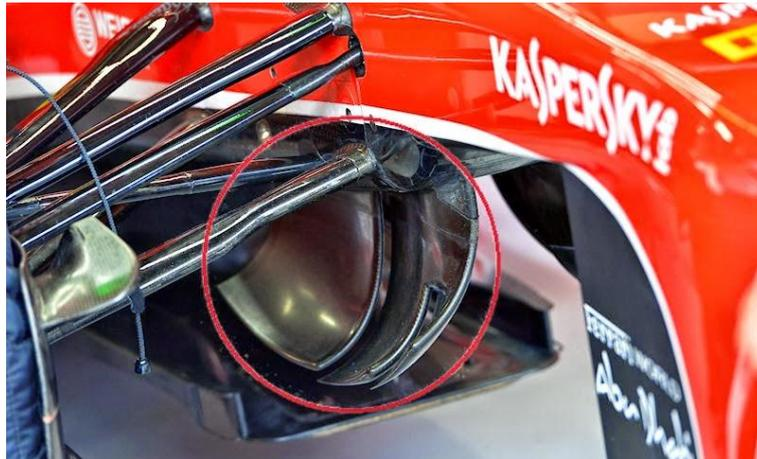
Fig 69. Turning vanes Ferrari. [9]
