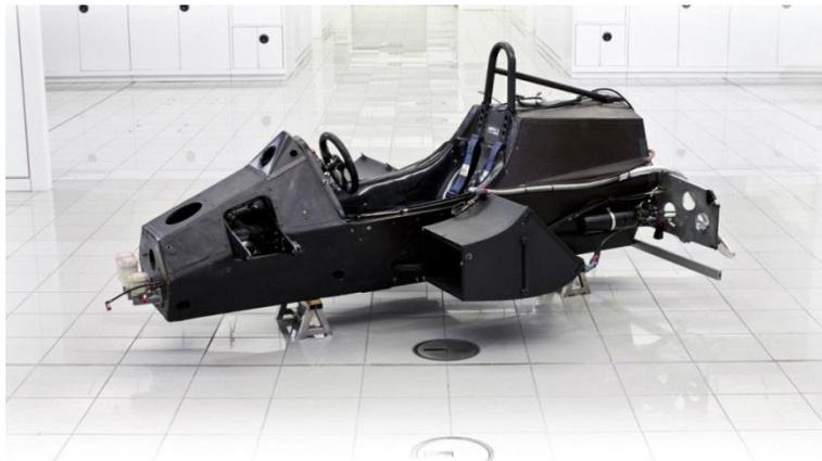
Fig 16. Chasis monocasco McLaren de fibra de carbono. [GP Library]
