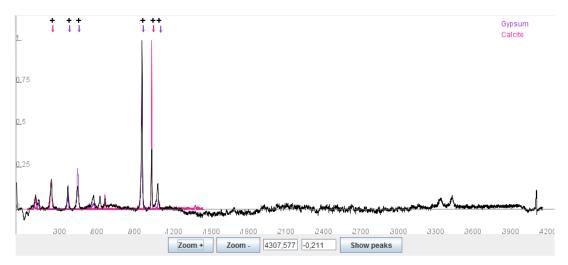
Figure 5.3: Mixture of calcite and gypsum.
