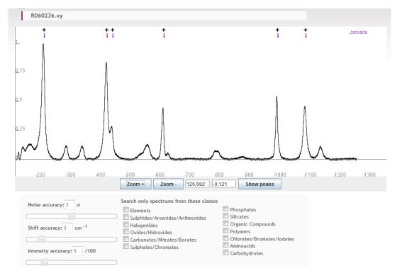
Figure 5.1: Example identification of a jarosite spectrum through the developed system.
