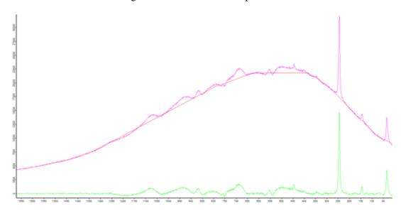
Figure 2.3: Baseline removal of magnetite spectrum.
