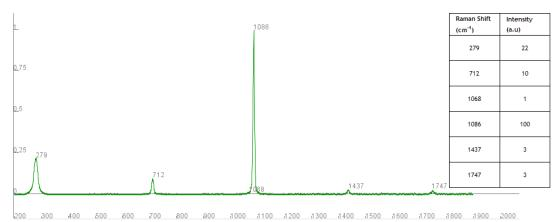
Figure 2.2: Calcite raman spectrum.
