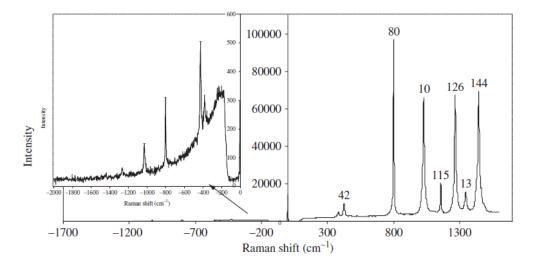
Figure 2.1: Stokes and anti-Stokes scattering for cyclohexane. To show the weak anti-Stokes spectrum, the y-axis has been extended in the inset.
