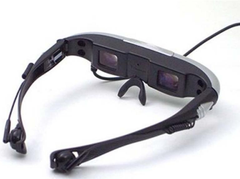
Figura 3.- Foto de un HMD (Head-Mounted Display) real [35]
