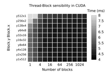
Figure 3: Effects of the Gang Number, Worker and Vector Length in the measured execution time using CUDA. Execution time is in milliseconds (lower is better). Darker is lower. Brighter is higher.
