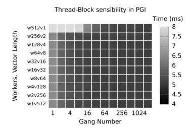
Figure 4: Effects of the Gang Number, Worker and Vector Length in the measured execution time using PGI compiler. Execution time is in milliseconds (lower is better). Darker is lower. Brighter is higher.
