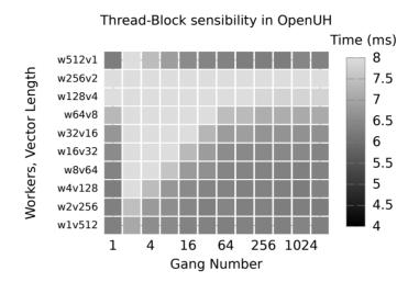
Figure 5: Effects of the Gang Number, Worker and Vector Length in the measured execution time using OpenUH compiler. Execution time is in milliseconds (lower is better). Darker is lower. Brighter is higher.
