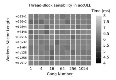
Figure 6: Effects of the Gang Number, Worker and Vector Length in the measured execution time using accULL compiler. Execution time is in milliseconds (lower is better). Darker is lower. Brighter is higher.
