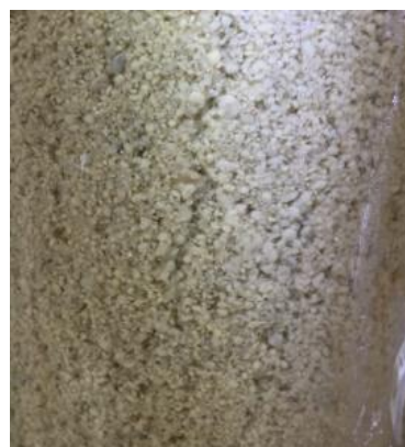
Figure 9 R4 on day 563 since the start-up of the reactor. 1.68 g/L tryptone connected. A disintegration of granules was observed despite the total amount of tryptone probably because new biomass was being produced in form of fluffy materials.
