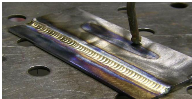
Figure 79: Welding seam in bronze. The surface in contact with the moving bracket will be covered in the same way where several layers will be applied (WeldingTipsAndTricks, 2018).
