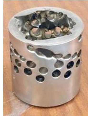
Figure 109: Erosion in a choke valve caused by sand (University of Southampton, 2018)
