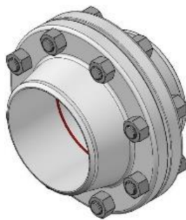
Figure 85: How the welded end flange will be connected to the pipeline using bolts and nut. (Wermac, 2018)
