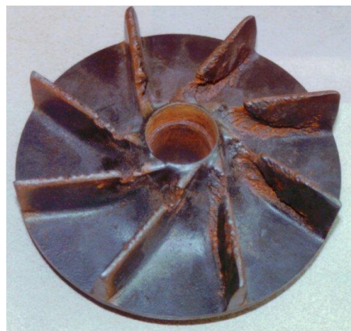
Figure 5: Damage on a pump due to cavitation effects (Schroeder, 2015).
