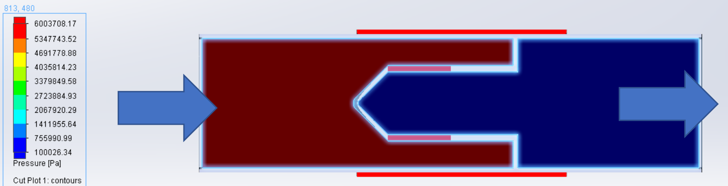
Figure 162: The pressure that will be used in the FEM analysis. The pressure on the left is 60 bars and on the right it is environmental pressure. The arrows indicate the direction of the flow
