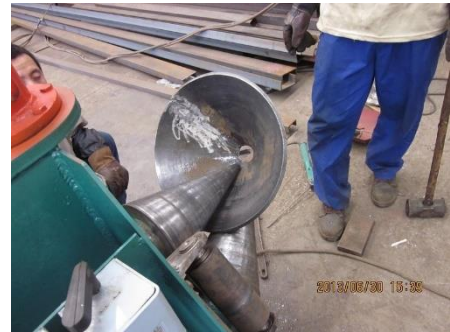
Figure 106: A plate roller bending a metal plate into a conical shape. The group sees roll bending to be the applicable production process for the front cone. (HB Machinery Co, 2013)
