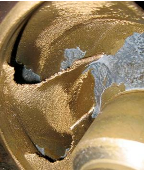
Figure 253: Turbine damaged by cavitation (MCOR, 2016)
